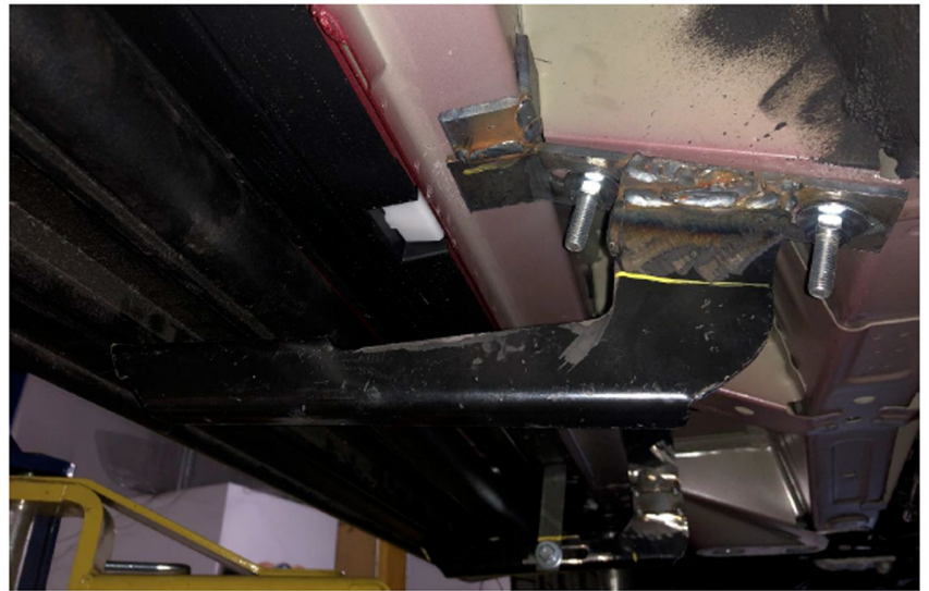
Picture shown with Driver Side Middle bracket with U-Bolt mounting
