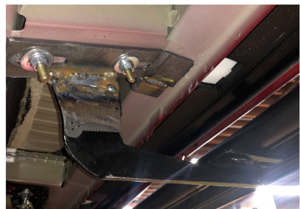
Picture Shown Driver Side Middle Bracket with U Bolt
